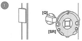
Thread the UNDER - ROSE [SR] in the protruding squared spindle [Q]. Fig.1
