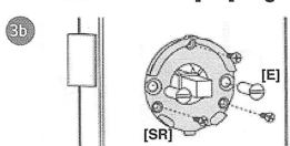
Only in presence of fitting kit-02 you will proceed by entering: N° 2 telescopic screws [P] into suitable holes located in the under-rose [SR] (lateral). Fig.3a. Above screws must be then properly tightened from other side by blocking the male part of telescopic screws [E]. Fig.3b
