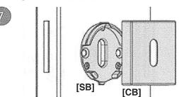
Place the UNDER - ROSE [SB] on the surface of the door and proceed by fixing it fastening the 3 retaining screws [V]. Fig.6
