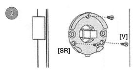
Use N° 3 retaining screws [V] to be fixed into relevant holes located in the UNDER - ROSE. [SR]. Fig.2
