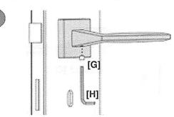
Apply the COVER- ROSE [CR] (already install on the handle) on the UNDER-ROSE [SR] by pressing. Fig.4
